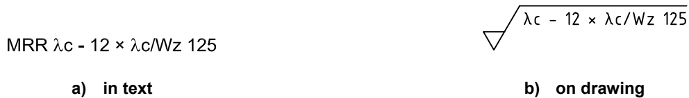
Figure 10 — Transmission band for waviness based on default cut-off \lambda_c for surface roughness
